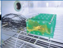
IMC is a critical layer that affects the reliability of the joint. This test studies the effect of high temperatures on the IMC
