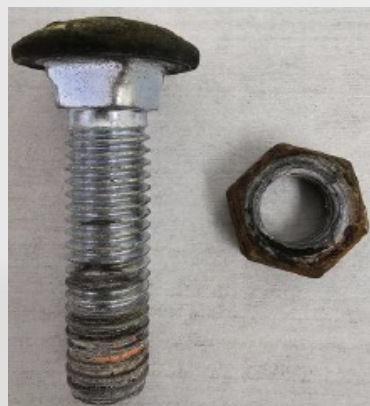
Corrosion on bolt/nut used for MSB
